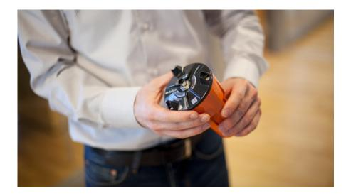
Glowing, burning or overheated products is the first indication of a beginning problem in the oven. Firefly BakeScan<sup>™</sup>-solution is designed to detect overheated, glowing or burning products on transport bands of baked products being transported out from the oven, for example biscuits, tortillas, baked crisps, bread and cereals.
