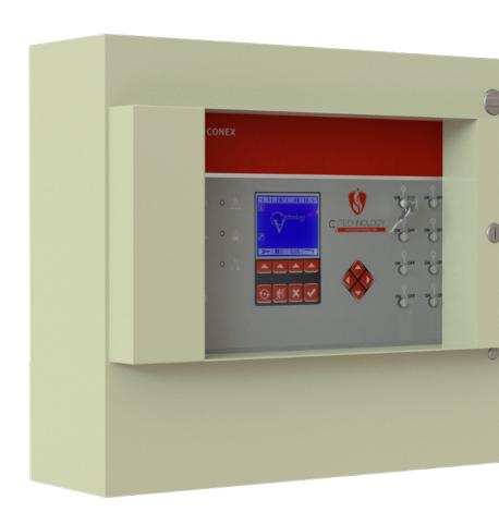
The controller features the ability to operate up to two independent operating zones at a time. A user interface is provided by a LCD screen, push button navigation, and signaling lights on the front of the controller enclosure. The interface includes a searchable data log and electrical lockout key switches for each zone. Six programmable dry contact relays are provided by the controller to signal for actuation, faults, or other operational states.
